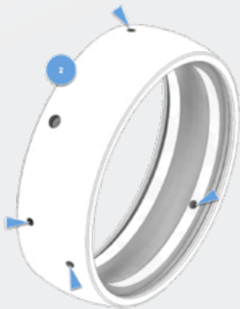
System G2: Outer ring with 4 lubrication holes in 2 lines
